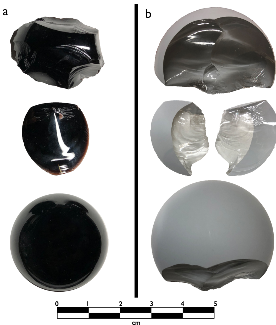
Figure 7. Manufactured glass hemispheres, including “black” glass and (a) spray-painted clear glass and (b) hemispheres and flakes made from each ( center left and center right ).
